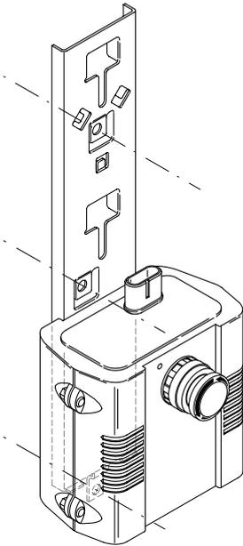
Mount the control unit in the 3 holes provided on the system carrier (→ fig. 2).
